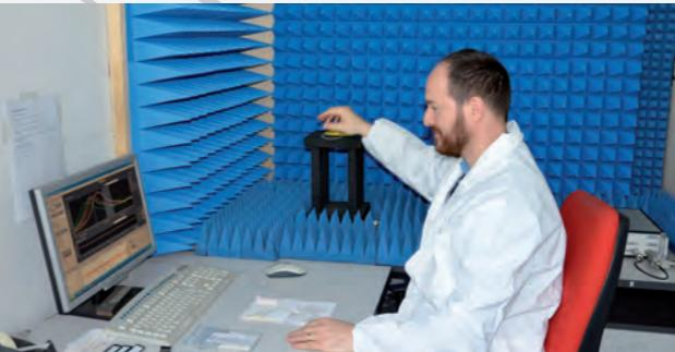
Smartres Lab is equipped with modern tools to check the tag response characteristics to the RFID activation field both in HF (High Frequency, today also for NFC, Near Field Communication and UHF, Ultra High Frequency).
